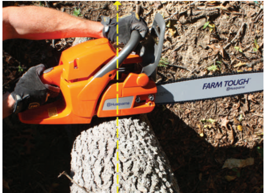
Many of today's chainsaws come with felling marks. Similar to the sight on a gun, these lines will help the operator align the cut in the direction the tree will be felled.
