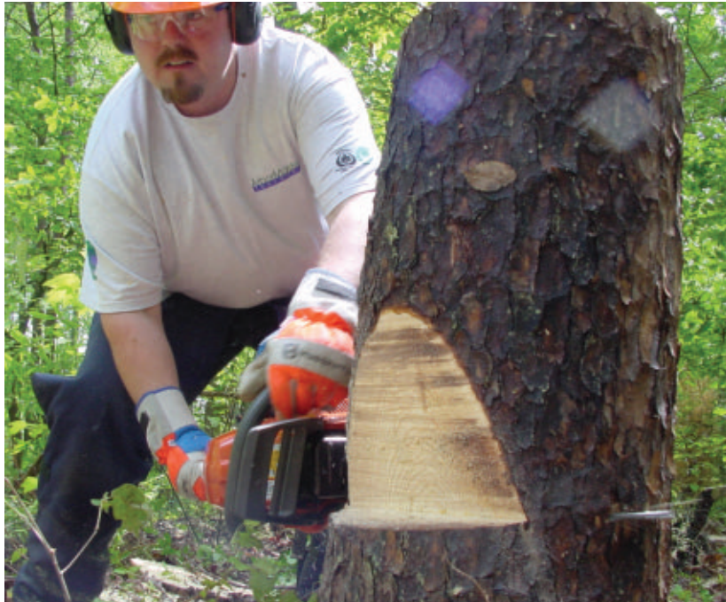
A 70-degree open face notch gives the cutter more control than a conventional 45-degree notch to make directional felling easier.
